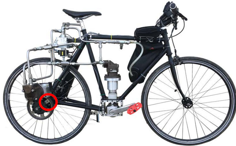
Figure 45b: Hall effect sensor mounting for vehicle speed measurement (red circle). The hall effect sensor mounted to the rear motor housing and takes advantage of a pre-existing bolt location for minimal additional hardware.
