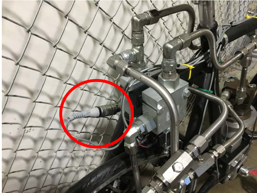
Figure 53: Rear view of assembled bike showing the location and mounting of pressure sensor (circled in red).
