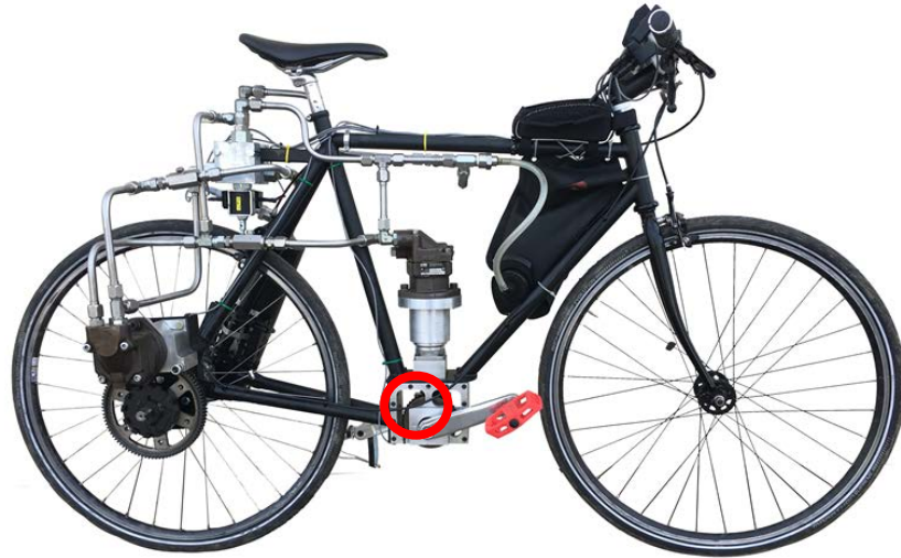
Figure 45a: Placement of hall effect sensor used for cadence measurement (red circle). The hall effect sensor is placed inside of the crank housing and allows for minimal invasiveness while the rider is pedaling.
