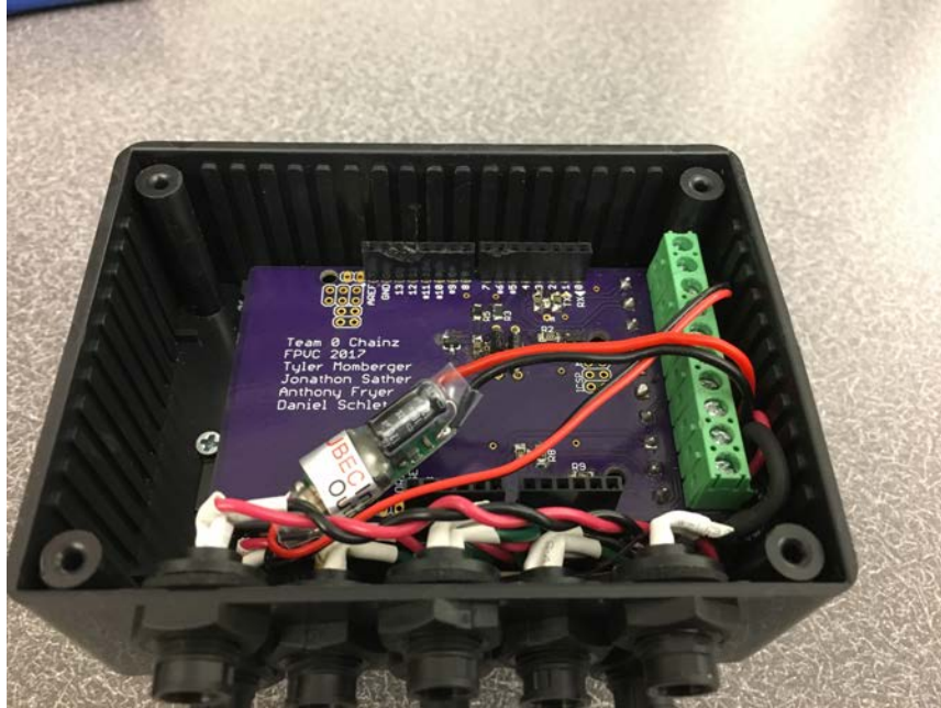
Figure 47: Assembled custom PCB in our display housing. The heatshrink package sitting on top is the buck converter, which steps down the 12V power to the 5V power used for the logic circuit.
