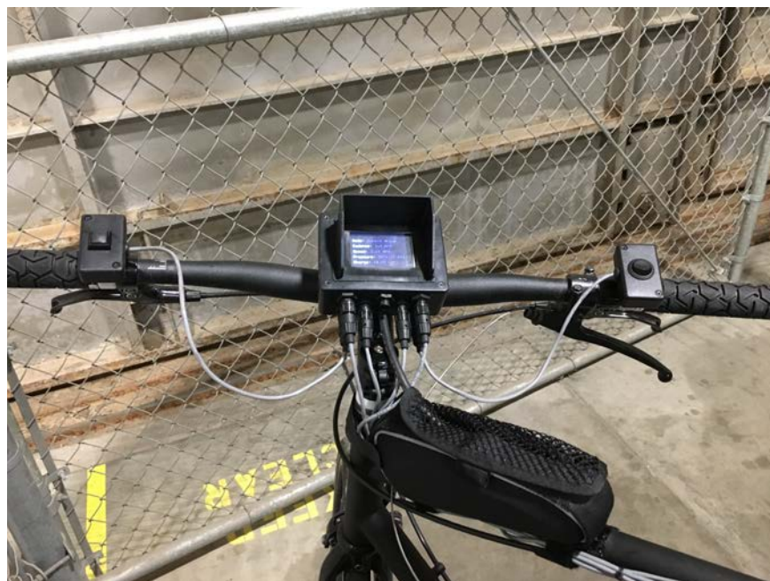
Figure 52: Display and switch assemblies mounted on the 2017 bike.
