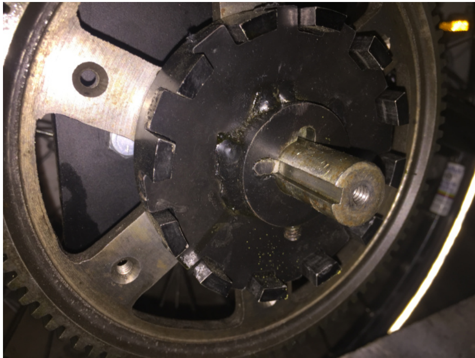
Figure 41: Clutch “fix” using keyway. Note that this eliminates freewheeling capabilities, but allows us to attain our goal accumulator pressure.
