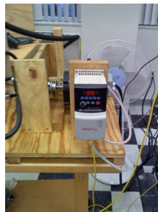
Figure 5: VFD for Motor Control
