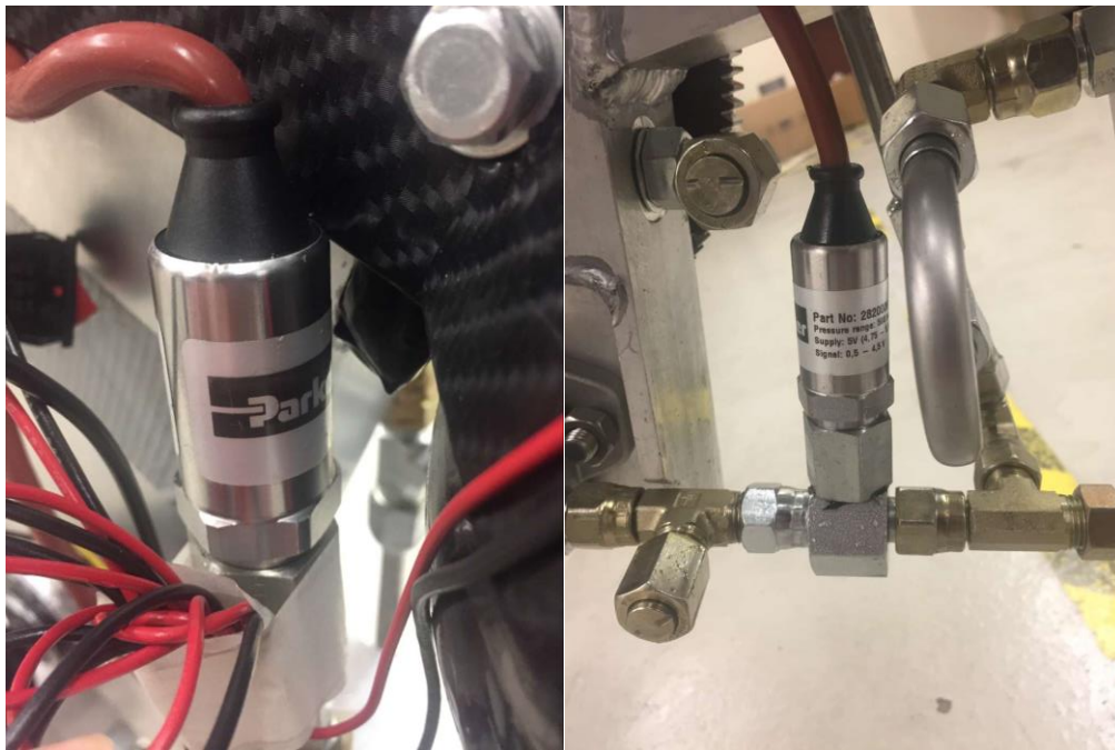
Figure 4.3.10: Pressure Sensor(Accumulator: Left / Main line: Right)
