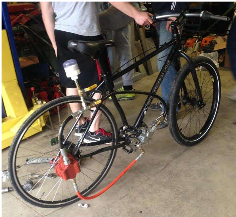
Photo 6: Direct Drive Assembled on Final Frame
