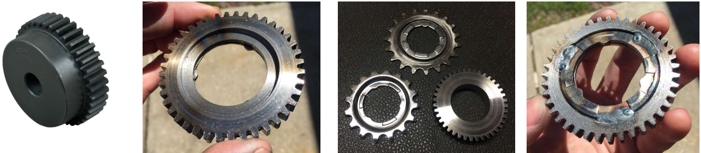
Photo 2: Drive side Gear - Machine to Weld
