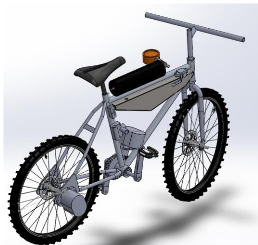
Figure 13: Updated Concept Design with New Pump and Motor
