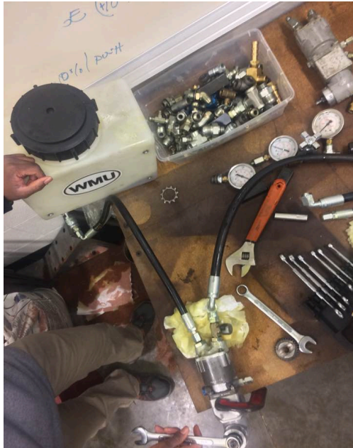
Image 19: Pump/Motor manual test
