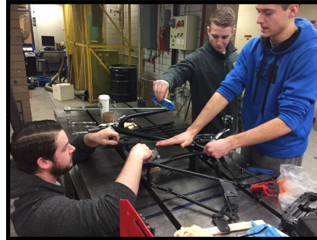
Frame Leveling (pre-weld)
