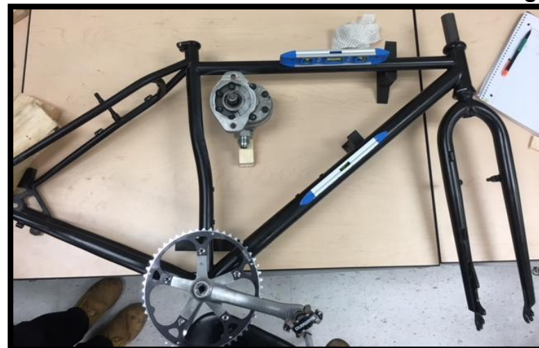
Initial frame leveling w. Pump
