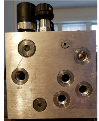
Figure 11 Manifold Motor, Pump, and Accumulator Ports
