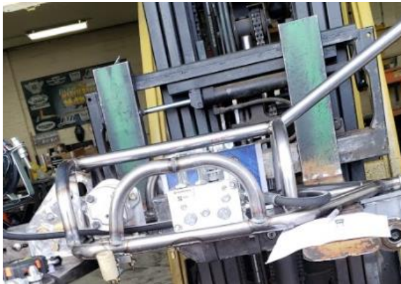
Figure 28. Tubing for Hydraulic Circuit by Hose Connections. Hammond, IN, 2020
