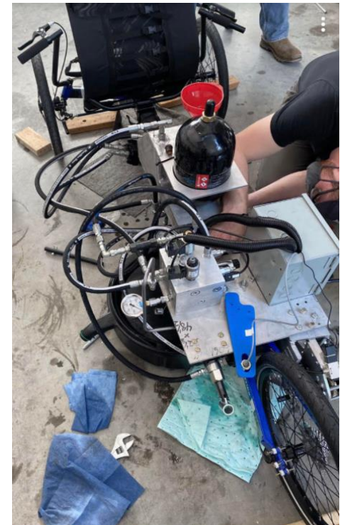
Initial tests using hydraulic lines, to ensure circuit works
