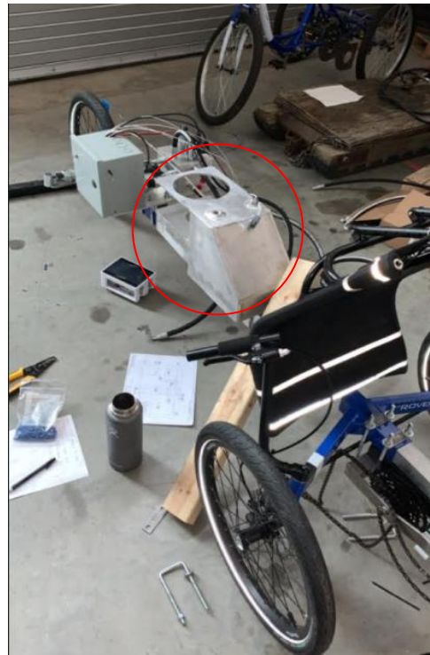
Wiring and initial chain routing
