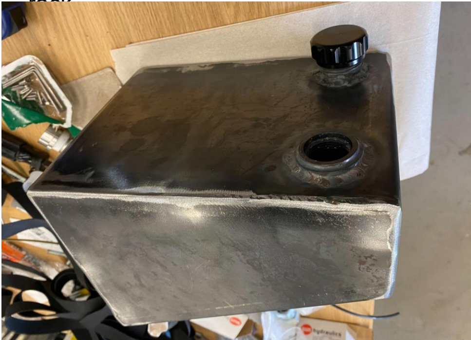
Custom hydraulic tank and rear
