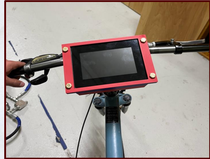
Figure 16. eX705 HMI mount CAD (left) & mounted unit (right)
