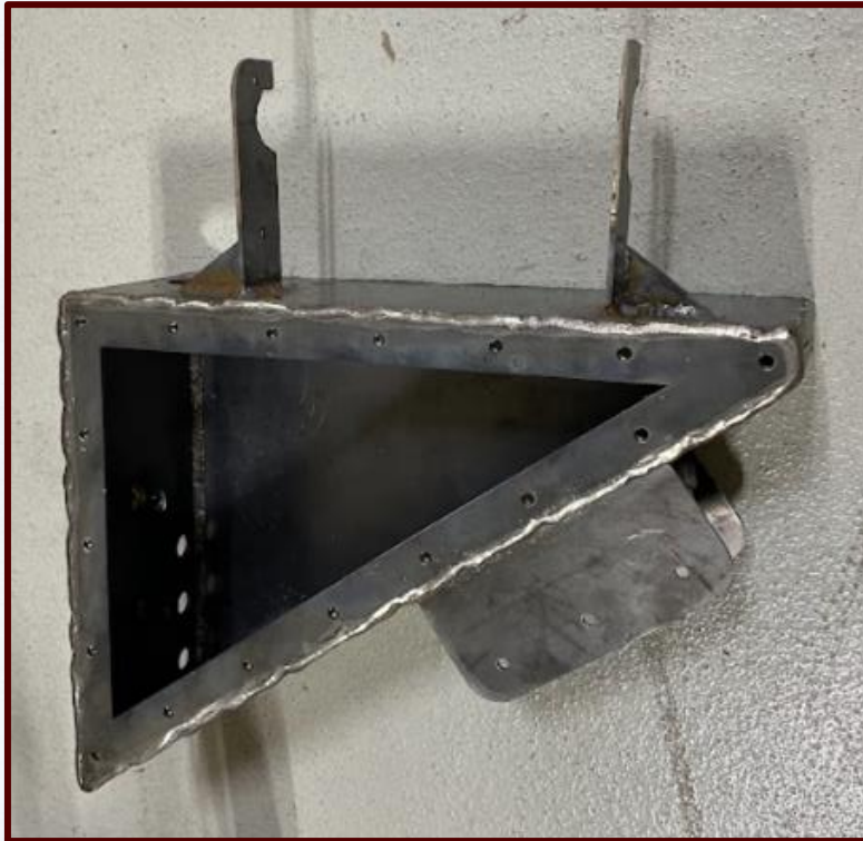
Figure 22. Welded reservoir (vertical baffle not shown) (Rust-Oleum clear-coat to prevent corrosion)
