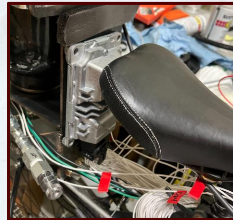
Figure 17. HY-TTC 32-CD-00-000 PLC (left) & mounted PLC (right)
