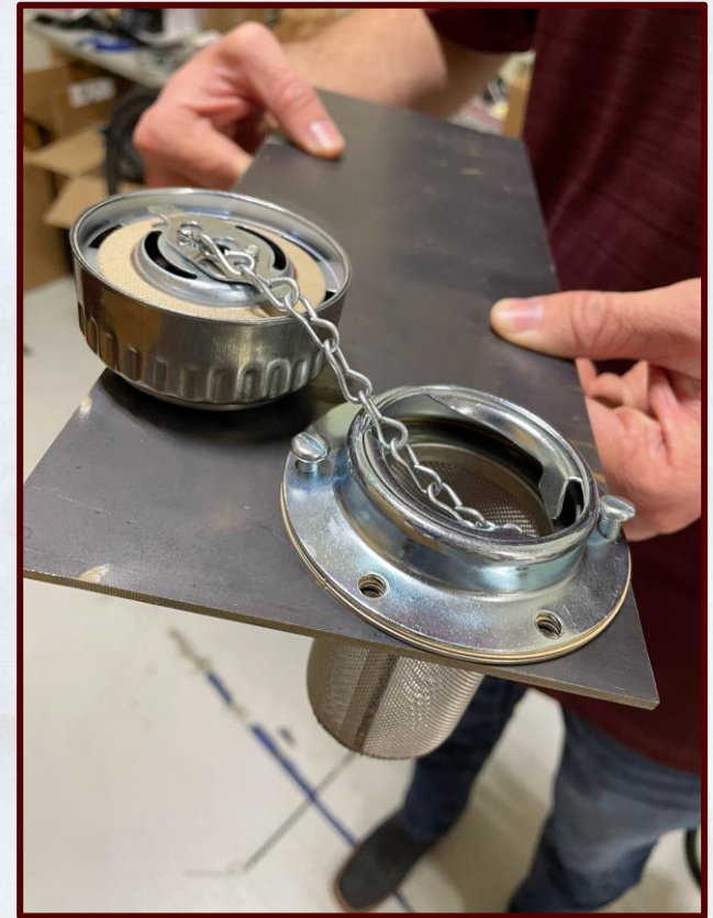
Figure 21. Vented reservoir fill port
