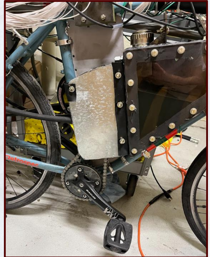
Figure 25. Bicycle main triangle assembly w/ chain guard
