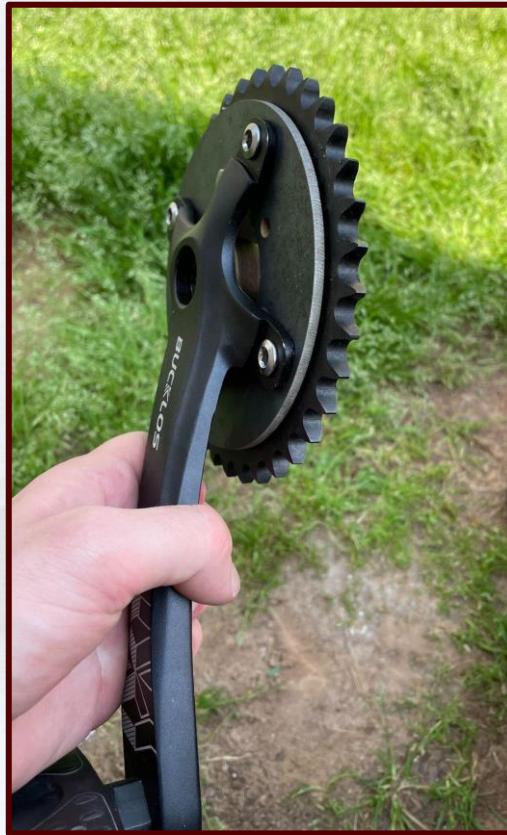
Figure 20. Crank arm w/ adaptor plate to #40 sprocket
