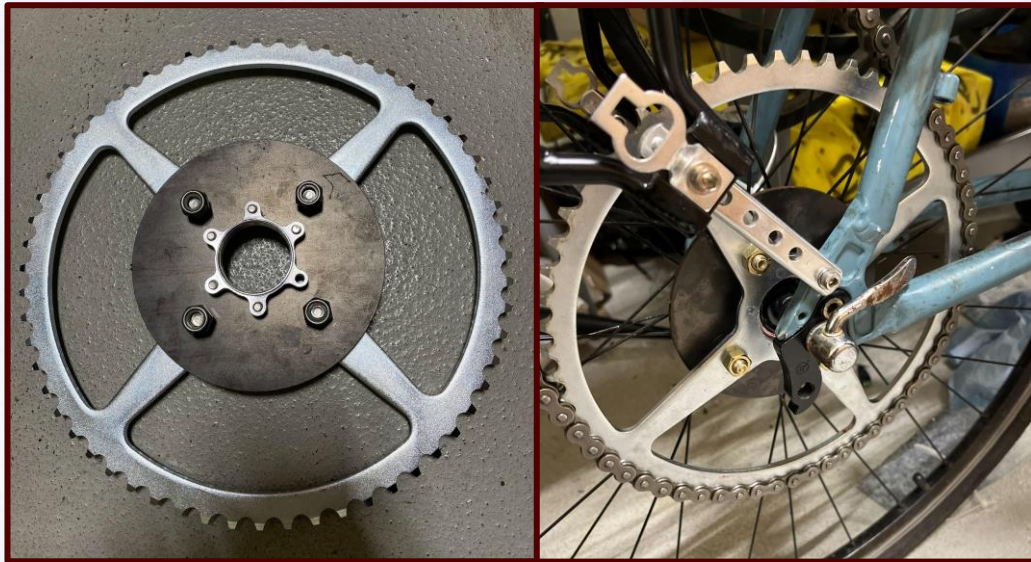
Figure 24. 60T 420 sprocket w/ adaptor plate to free wheel thread
