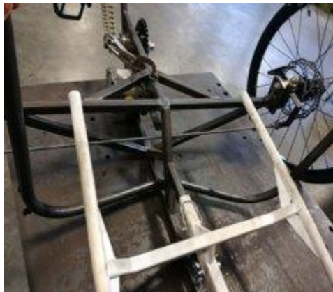
Fixed dual drag link to the front wheels
