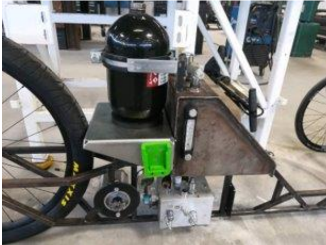
Mounted accumulator behind reservoir
