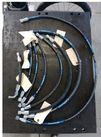
Installing hoses to the hydraulic components
