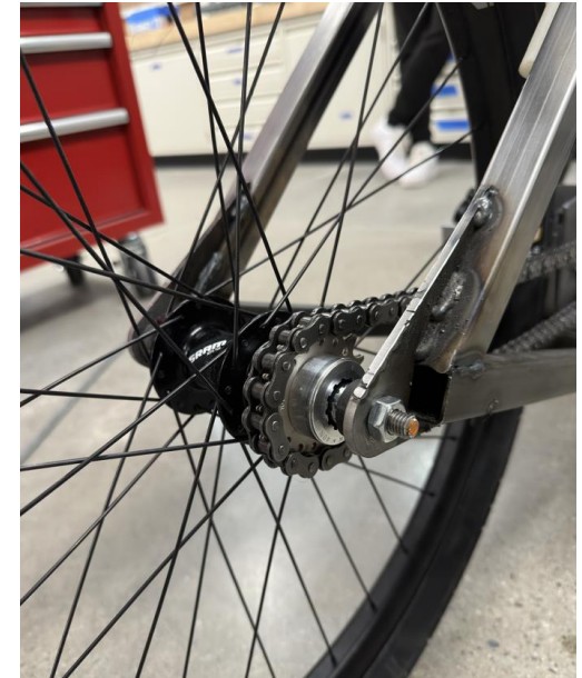
New back wheel, axle, and sprocket
