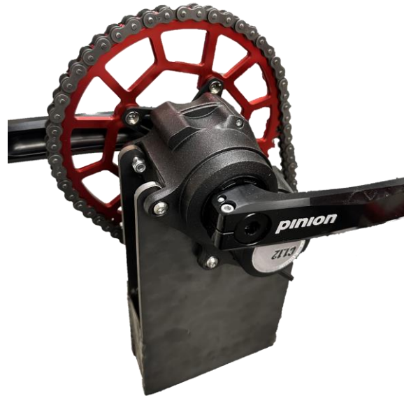
Incorporated a 12 speed Pinion Gearbox
