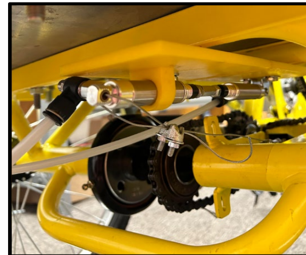
Cylinder Assembly Installed
