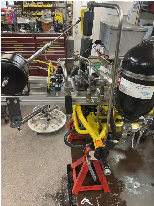
Hand pump replacing the manifold
