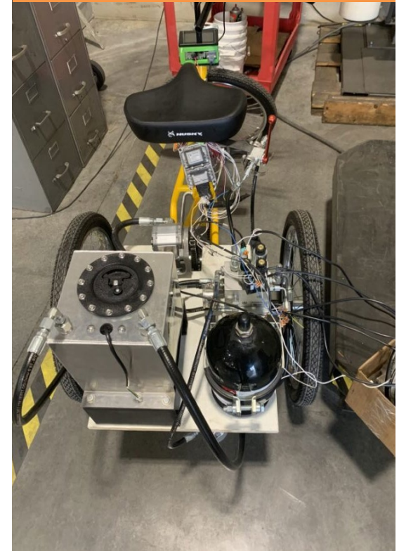
Installation of HMI and Wiring
