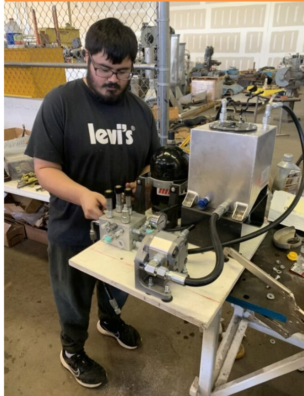
Installation of Hosing, Valves, Transducers, & Gauges
