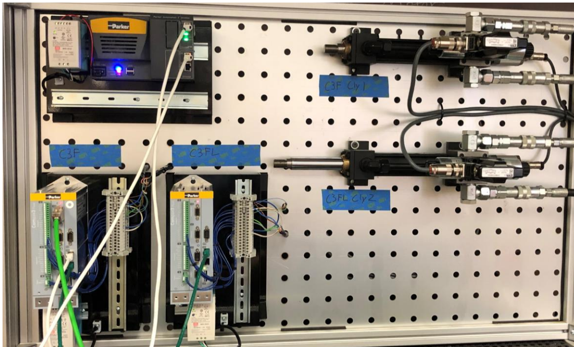
The Setup with PAC Controller and Two EH Station
